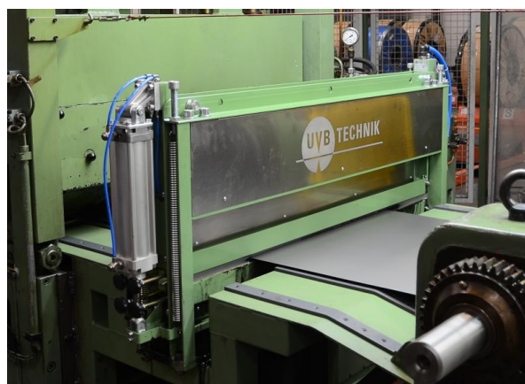
Fig. 7: Wiping equipment on the cut to length line
