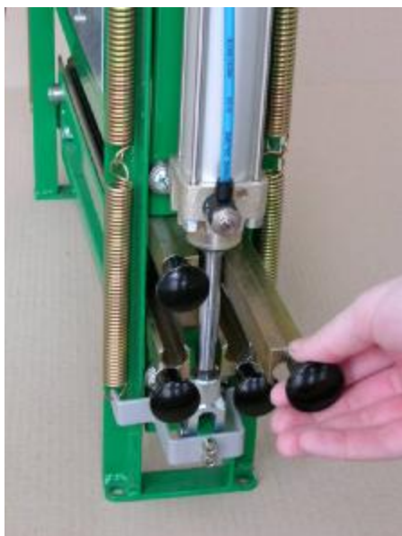
Fig. 2: Side movement of slat holder while the slats are changed
